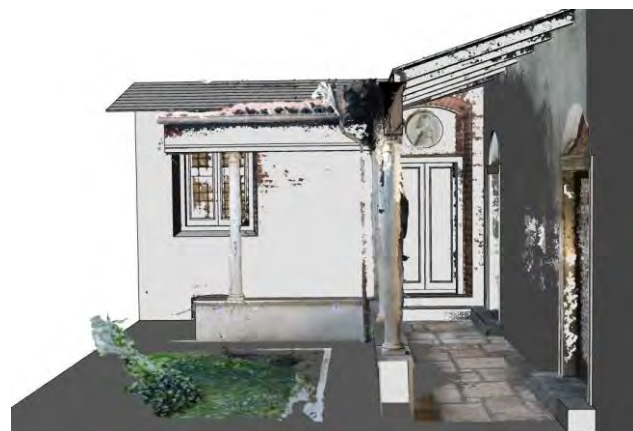
Figure 7. Mathematical reconstruction starting from the mesh
