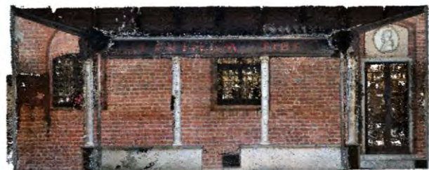
Figure 6. Pointcloud of the western wall of the cloister
